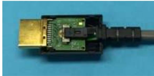
Figure 2: Interior of AOC End Module
